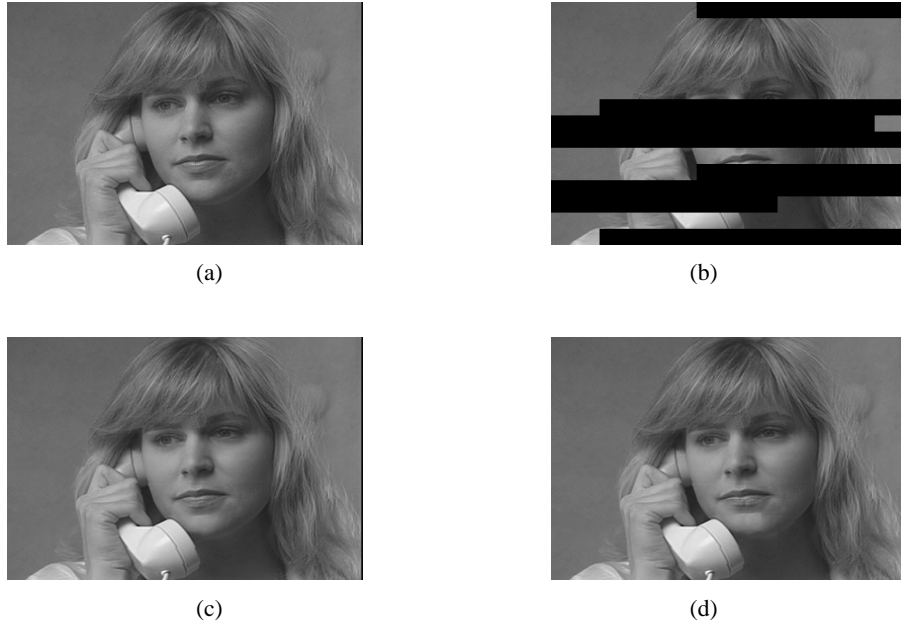
Fig. 7. Error concealment performance of different algorithms for frame 120 in the 'Susie' sequence. (a) Original/error-free, (b) with packet-loss artifacts (PSNR=10.435), concealed with:(c) two-line search SMA (PSNR = 34.25)and (d) SAA (PSNR=34.17).
